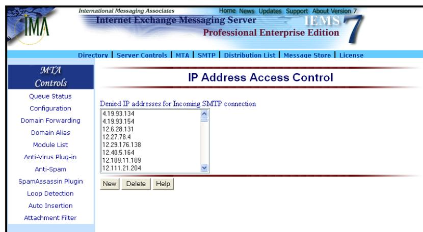
Figure 35: Adding and Deleting Banned IP Addresses
