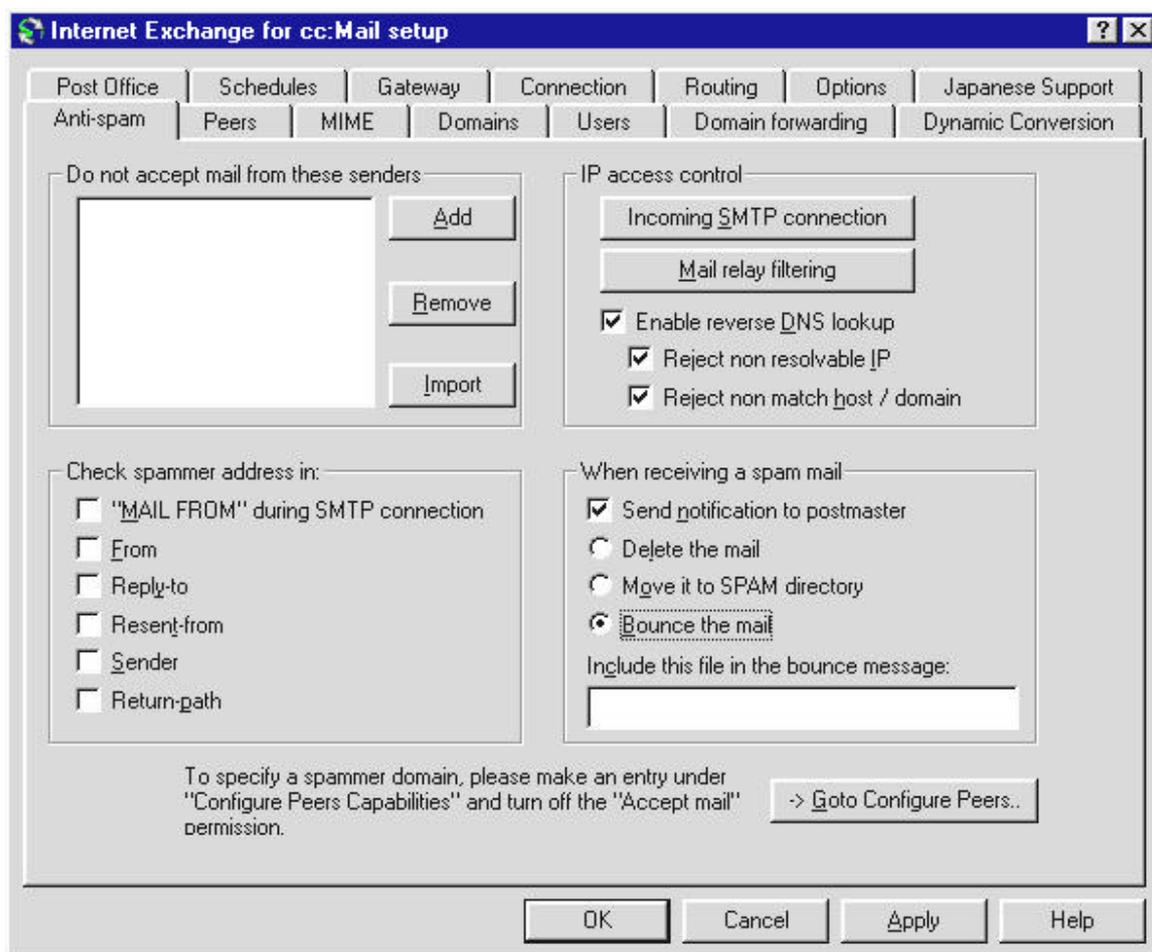
Figure 5. GUI for activating **Enable Reverse DNS Lookup** option
